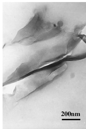
Fig. 3. TEM images of PPC/OMMT nanocomposites with 4 wt% OMMT content.
